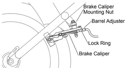
To tighten the cable, loosen the lock ring and turn the barrel adjuster in the counter clockwise direction. Secure the barrel adjuster in the new position by tightening the lock ring against the caliper or brake lever body.
