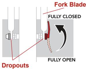
While maintaining the wheel in this position, rotate the quick release upward and into the FULLY CLOSED position. When properly closed, the curve of the quick release will be pointing toward the wheel and parallel to the fork blade. To generate enough clamping force it is necessary to wrap your fingers around the fork blade while closing the quick release lever. The proper force required to close the quick release lever should leave a visible imprint in the palm of your hand.
