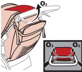
After installing Weather Shield, confirm vents on Weather Shield are aligned with space above seat back and all other vents are free of obstruction.
