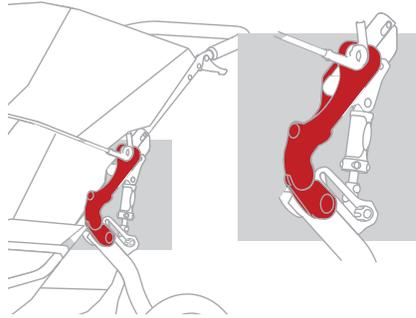
Attaching BOB accessories is simple and easy with this push button, lock and release design. The accessory adapter also allows for many accessories to remain attached when the stroller is folded. See Stroller Accessories section of this manual for more information on all available accessories.
