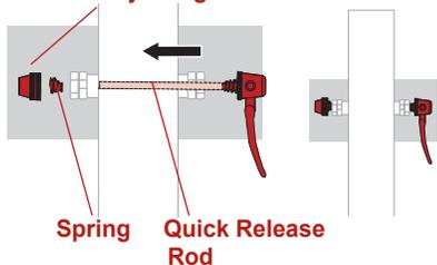
**NOTE:** Prior to installing the front wheel it is necessary to open the brake quick release to provide clearance for the wheel/tire to pass the brake pads.
